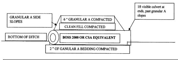
INSIDE BOTTOM OF CULVERT TO BE AT SAME GRADE AS EXISTING DITCH BOTTOM OR AS DIRECTED BY MUNICIPALITY
